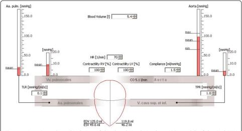
Figure 2 An animated graphical view of the closed circulation loop (CCL model) of the CLabUZH software, including the listboxes controlling the input parameters and the manometers displaying current pressure values. Abbreviations: arteriae pulmonales, Aa. pulm.; heart rate, HR; left ventricle, LV; right ventricle, RV; end-diastolic volume, EDV; end-systolic volume, ESV; total peripheral resistance, TPR; total lung resistance, TLR.
