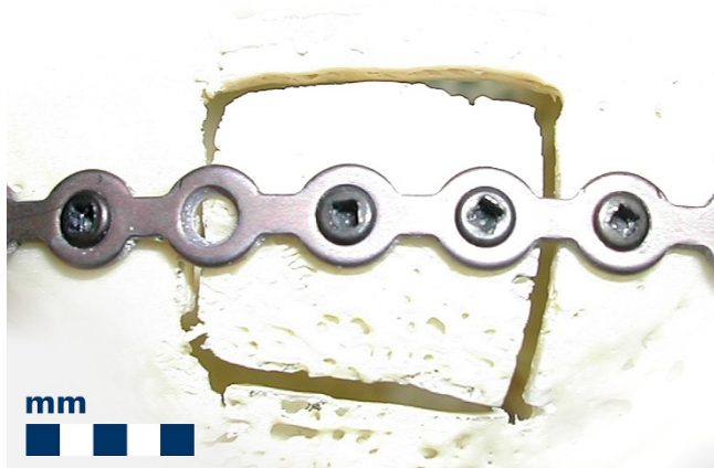
Figure 1 Conventional fixation of an osteosynthesis plate with screws. The conventional fixation of an osteosynthesis plate on a rabbit bone sample with a square cut damage of ca. 1 cm 2 as it is common in midfacial surgery. The plate is fixed to the bone by fastening screws in the osseous lamella to both the bone of sufficient cortical bone mass and to the fragile bone fragment.
